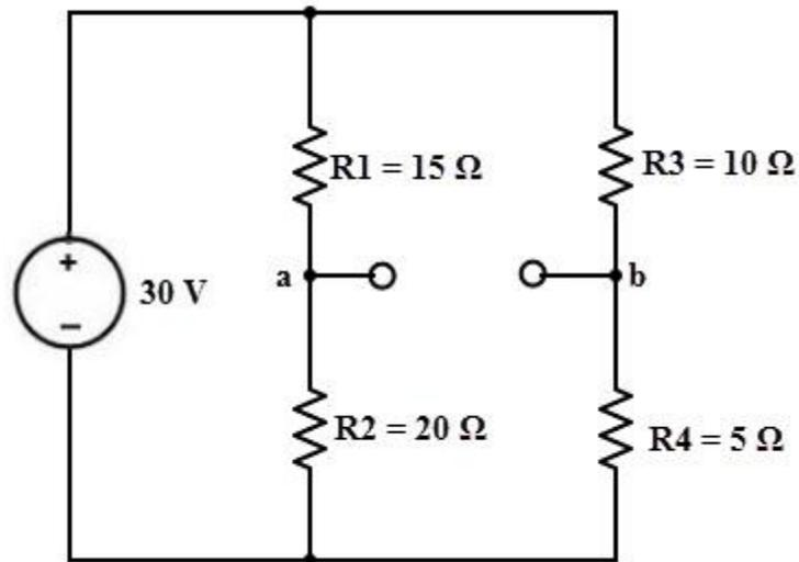
The Thevenin's voltage or voltage across the terminals ab is  $V_{ab} = V_a - V_b$
