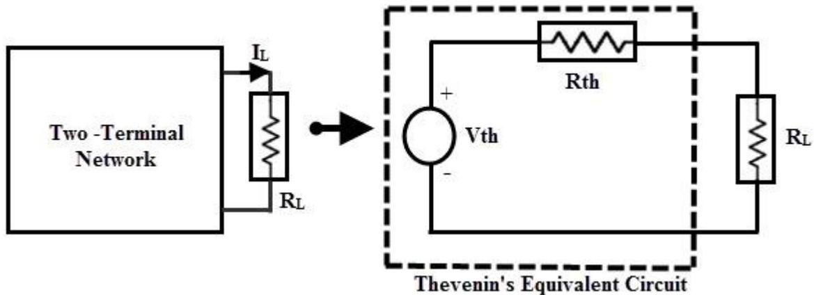
The original two terminal network is replaced with a Thevenin's equivalent circuit across the variable load resistance. The current through the load for any value of load resistance will be
