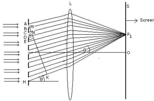
Figure (1) Fraunhofer diffraction at a plane transmission grating
