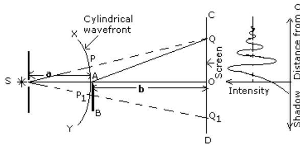
Figure (1): Diffraction at a straight edge
