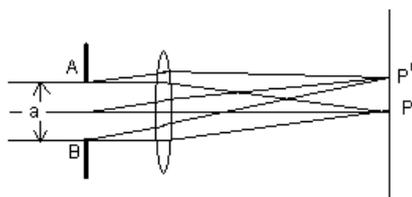
Figure (1) Diffraction at a single slit.
