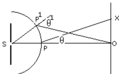
When  $\theta = 0$ , the wave move along the normal to the wavefront along PO and hence the zone around P has maximum effect at O
