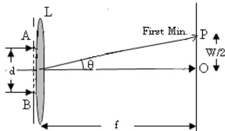
If the lens is placed close to the slit, then the distance between the slit and the screen is ‘f’.
