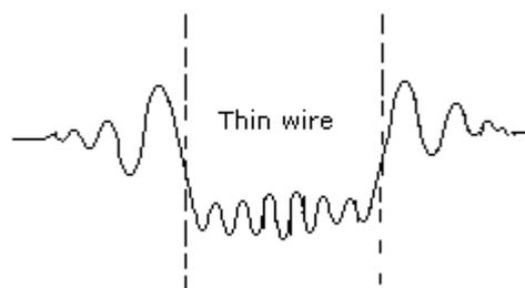
Figure (2): Intensity distribution in the diffraction pattern on a thin wire.
