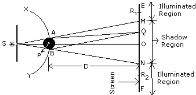
Figure (1) Fresnel diffraction at a wire
